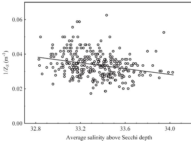
Fig. 6. Relationship between the reciprocal Secchi depth ( $1/Z_S$ ) and salinity for the stations where average Chl  $a$  above Secchi depth was lower than  $0.1 \text{ mg m}^{-3}$ . The slope of the fitted regression line is  $-0.008 \pm 0.003 \text{ m}^{-1}$  per unit of salinity ( $\pm \text{CI}$ ) ( $p < 10^{-5}$ ,  $n = 314$ ). For these low Chl  $a$  concentrations there was no significant relationship ( $p > 0.05$ ) between reciprocal Secchi depth and the Chl  $a$  concentration.
